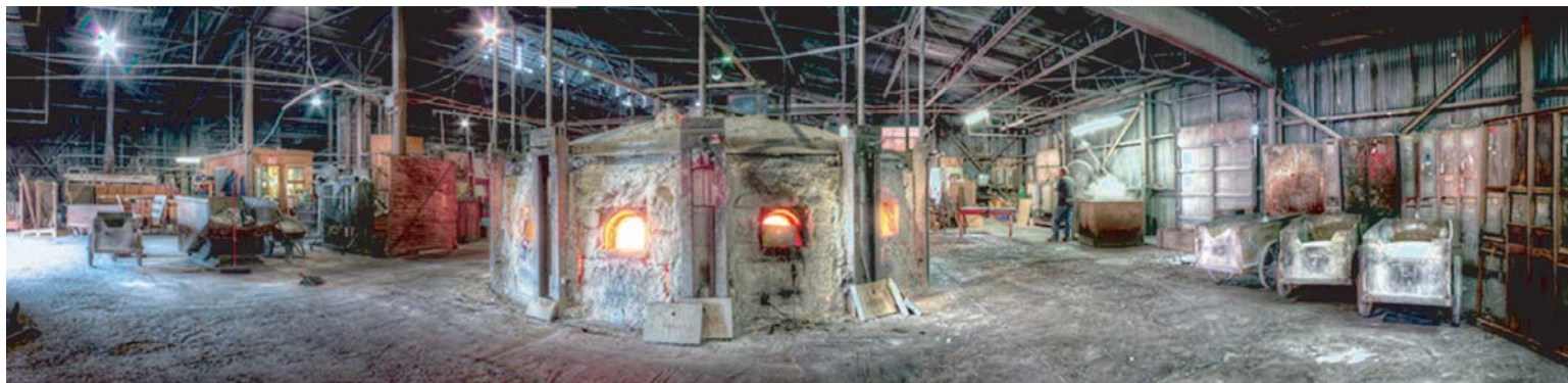
Panoramic image of the Kokomo Sheet Glass Shop, with the 12 pot furnace known as "The Beehive" in the center.
